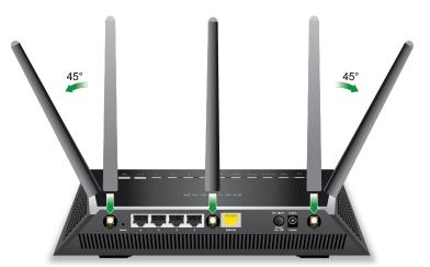
We recommend that the center antenna be vertical and that you aim the others outward at 45-degree angles, as shown.
